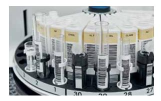
analyzer is as well a good example for efficient, highly developed design. The respons®910 is the only analyzer in its class with a multifunctional arm that integrates clot detection and crash sensor, liquid-level detection and pipetting of sample and reagent. The instrument is user-friendly as well since all components are almost maintenance-free.
